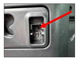
The use of long nosed piers or a magnet will make removing the fixings easier from this location. Set aside the 2 x fixings with the hooks and shelf supports and their fixings. These can be re-installed should you wish to remove the boot basket in the future.
