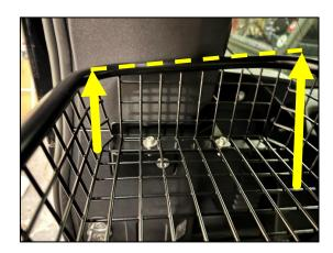
Secure the basket to the support brackets using the 4 x M6 x 15mm cap head fixings.
