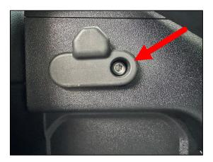
Hinge the fold out 'coat-hooks' downwards to approx' 45-degrees and then pull on the hook upwards to unclip the coat-hooks from their housing.
