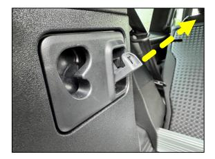
With the coat-hook removed this will reveal the TX27 Torx fastener located within the coat hook location. Remove this fixing.
