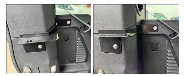
The 2 x longer M6 x 60mm cap-head bolts are used for the rearmost fixing points on the support bracket.
