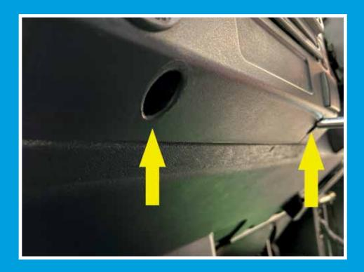
Loosen the three screws across the top of the radio console. You DO NOT need to remove these screws completely since you'll notice the three plastic locating tabs on the top of the console are slotted. The fixing screws clamp down on these slotted tabs. With the screws loosened you can now pull the console clear of the dashboard and begin to disconnect the radio, switch connections etc.
