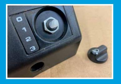
If you don't have a headlamp levelling switch, simply transfer the blanking plug across to the Double DIN
