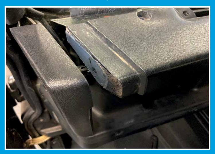
With the dashboard top rail removed you can now see how the original centre console is fixed in place. It is held in place with a total of five screws. All of these fixing screws will be reused when installing the MUD Double DIN Console.
