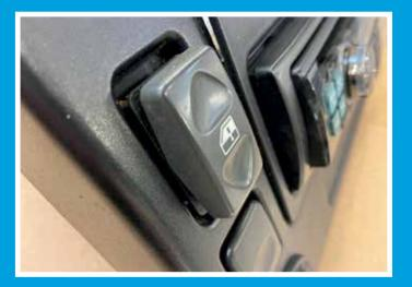
Remove the full width switch retainer housing from the back of the original radio console and transfer over to the MUD Td5 Double DIN Console. Secure to the Double DIN Console by reusing the original screw fixings. Refit the switches into the MUD Td5 Double DIN Console in their respective locations.
