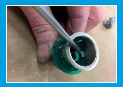
It is very common for the plastic bulb holder to have become hard and brittle over time due to the heat generated by the bulb. This normally results in the locating tabs breaking when you try to release them. Providing the earth contact on the bulb holder maintains contact with the body of the 12v socket, a wrap of insulating tape to hold the bulb holder to the socket will ensure the socket will continue to illuminate.
