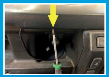
Prise out the oval Land Rover insert from the passenger side grab-handle to reveal the fixing screw underneath the insert. Remove this screw. Remove the lower fixing screw.
