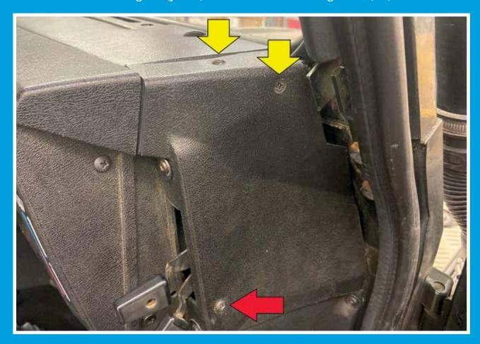
Carefully pull the binnacle and heater control assembly away from the dashboard just far enough to clear the dashboard top rail. You do not need to disconnect any of the electrical connections.
