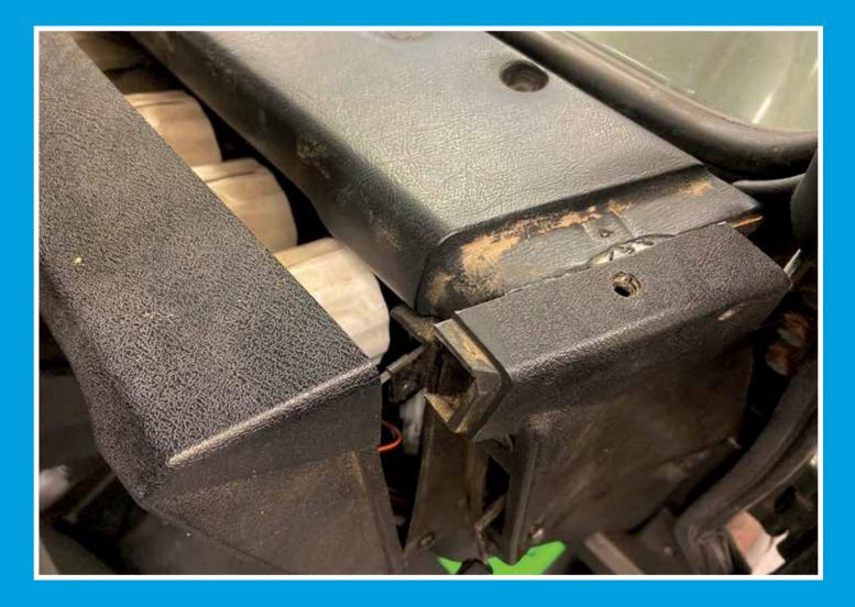
Locate and remove the two concealed screws that go upwards into the dashboard top rail to either side of the radio console.
