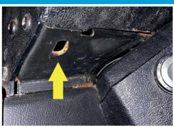
Remove the heater control fixings  $x \ge (yellow)$  and loosen the lower fixing circled (red).
