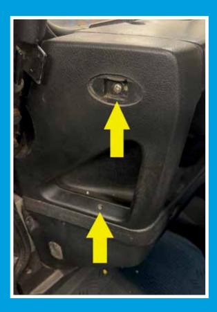
With the grab-handle fixing screws removed, the grab-handle will now lean outwards just far enough from the end of the dashboard to release the dashboard top rail.
